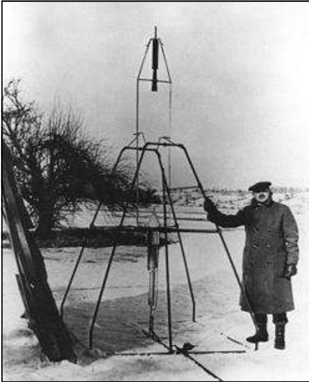
Robert Goddard, bundled against the cold New England weather of March 16, 1926, holds the launching frame of his most notable invention — the first liquid-fueled rocket.
